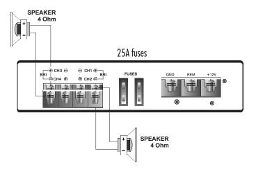
Note that the two speakers & four speakers have been connected to the four terminal following the (+) and (-) graphic. Your speaker terminal may be marked (+) and (-) or there may be red dot by one terminal which means the same as (+). Connecting the speakers in this manner assures that the two speaker cones will move in and out together according to the original recording. If one of the two speakers is reversed, stereo imaging and bass response will be degraded.
